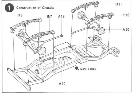
③ (Construction of Chassis and Body) Make sure of fixing A13 prior to the main assembly. Cement the pre-assembled chassis and body at ⑤ & ② together.
